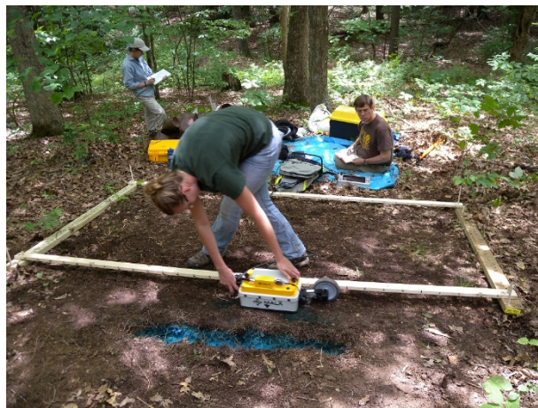
PHOTO: Geophysical survey of dye tracer test on the Shale Hills CZO conducted by Temple University.
